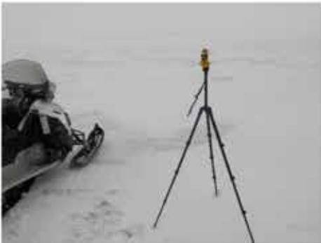
**Weather monitoring using the Kestrel 5500 Weather Meter**
